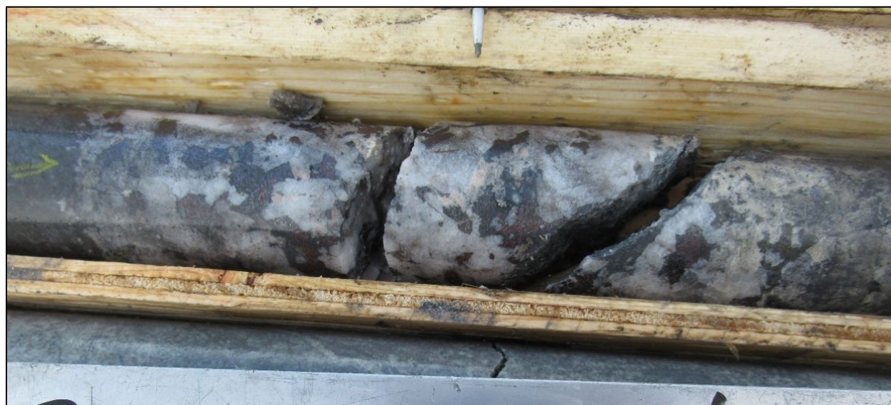
FIGURE 10.2 DRILL HOLE SQ20-010 INTERVAL CONTAINING 56,115 G/T AG OVER 30 CM
